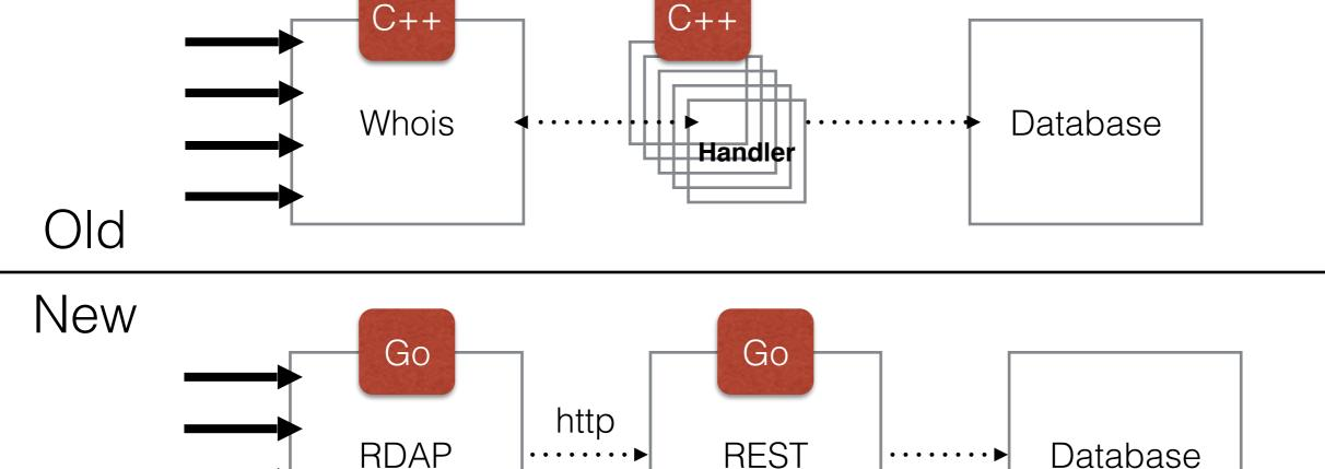
Go RDAP daemon works using a web service architecture and exchanges data with a REST backend
